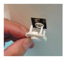
14-It may be necessary to reinstall the button assembly, (especially if the thermal switch is not centered.) This can be done without disassembling the unit. See "Button Assembly Instructions", (on website), if more instruction is required.
