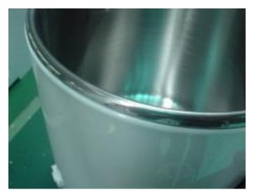
11-Insert the shell in the slotted rim of the stainless steel boiling chamber.
