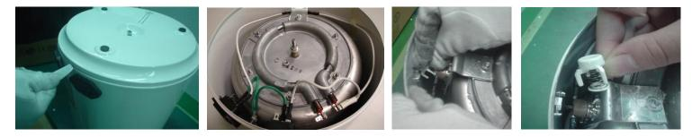
4- Use a thin screw driver to insert into the space between base and distiller body and remove the base.
