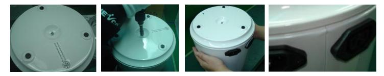
2-Remove the nut and lock washer. (Be careful not to scratch the surface) 3-Pat the outer cover to create a space between the outer covering and base cover.
