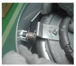
6-Slide the white wires off the thermal switch terminals.
