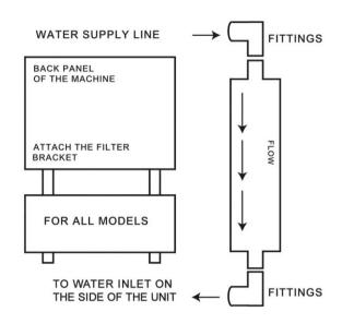
Attach the plastic line coming from the pre-filter directly to the inlet on the left side of the unit. Use Teflon sealing tape on threaded fittings. Push plastic line firmly onto the inlet and tighten.
